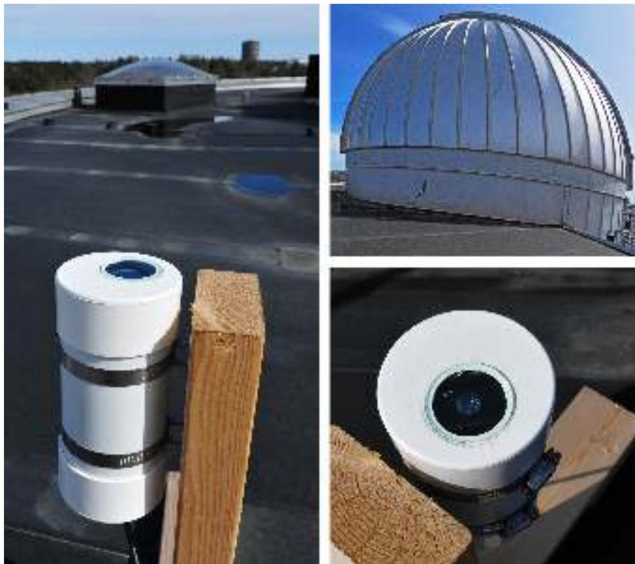
Figure 3: Sky Quality Meter mounted at the roof of Albanova University Center in Stockholm
